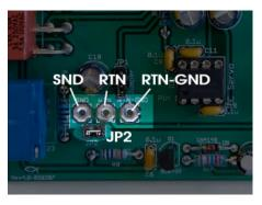
In normal operation, JP2 connects the SND solder pad to the RTN solder pad.
