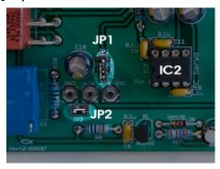
To facilitate easy setup, jumper terminals are used in the SC-1 Mic Preamp. There are (2) jumper terminals, JP1 and JP2. In normal use, both jumper terminals must be shorted and "jumpered."
