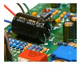
STEP 10: Solder the Bourns potentiometer. Make sure the component is flushed to the board. Solder the middle leg first, check alignment, and then solder the other 2 legs.
