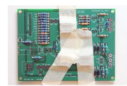
STEP 6: Solder the two jumper connectors, JP1 and JP2. Make sure they are soldered straight up, and not crooked to the left or right. TIP: Solder one leg first. Check if it is straight. Then continue soldering the other leg.
