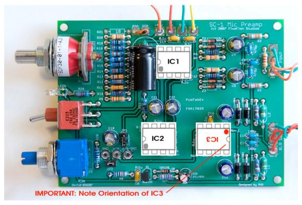
**IMPORTANT NOTE:** This is really, really important! IC3 is mounted in a different orientation from IC1 and IC2. Please observe this precaution and avoid mounting IC3 in the wrong orientation. Otherwise, you run the risk of damaging IC3. See photo above showing the correct way of how IC1, IC2 and IC3 are mounted.
