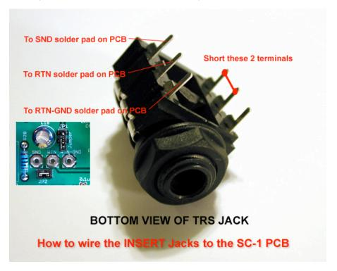
Do not forget to short the two terminals on the jacks. This connects the SND connection to the RTN connection completing the circuit if there is no TRS jack inserted.
