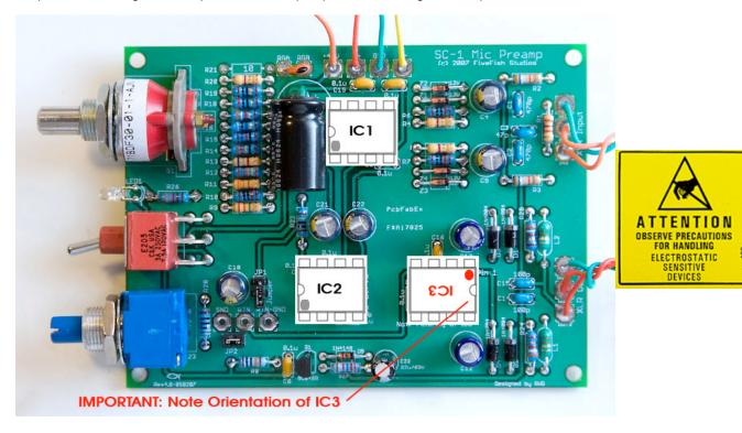
STEP 14: Solder wires to the +48V, +18V, GND, and -18V pads. Connect the wires to your power supply (or PSU-1848 If you also bought the PSU kit).
